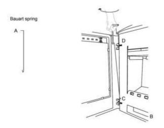
\*Tool for mounting the "Bauart" spring can be bought here
