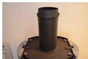
**5:** If you would like a top outlet then remove the cast iron branch piece on the top of the stove and mount the accompanying pipe, remember the gasket between the pipe and the stove. The cast iron branch piece is then mounted on the top of the accompanying smoke pipe, remember the gasket between the pipe and the branch piece.
