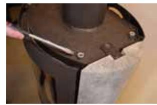
**3:** Remove the 4 or 5 nuts that are mounted on the top of the raw stove, do not discard them, they will be used under point 21
